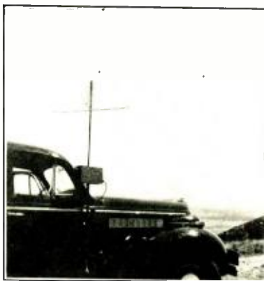
W6IOJ's ground-plane vertical antenna mounted on the side of his car. The oscillator-detector portion of his transceiver is mounted in the black box at the base of the antenna. The audio amplifier and modulator are inside the car.
