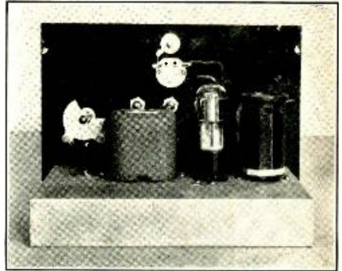
Figure 3. Removing the batteries shows the transformer, coil, tube, and condensers.
